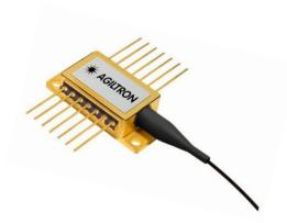
The 520nm series laser diodes are fabricated in a hermetically sealed 14-pin butterfly package. The laser diodes contain a monitor photodiode, thermoelectric cooler (TEC), and a thermistor to secure high-quality laser performance. The Laser Diodes Wavelength of 520±10nm, Output power: ≥10mW, Pigtail Type: 405-HP(Nufern) fiber with 900um loose tube, 1.0+/-0.1m, FC/APC connector. Our laser products are Telcordia GR-468 qualified and in compliance with RoHS Directives.
